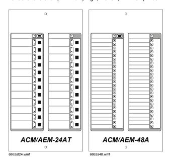
**AEM-24AT**: The Annunciator Expander Module-24AT expands the ACM-24AT by 24 system points. The AEM-24AT is identical in size and in frontal appearance to the ACM-24AT. Up to three of these expander modules can be supported by an ACM-24AT, for a maximum of 96 system points. 8.375" (21.27 cm) high; 4.375" (11.11 cm) wide. **NOTE:** The AEM-24AT cannot be used to expand the ACM-48A.
