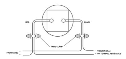
SSM24-X SERIES BELL WIRE CONNECTION (BACK VIEW)
